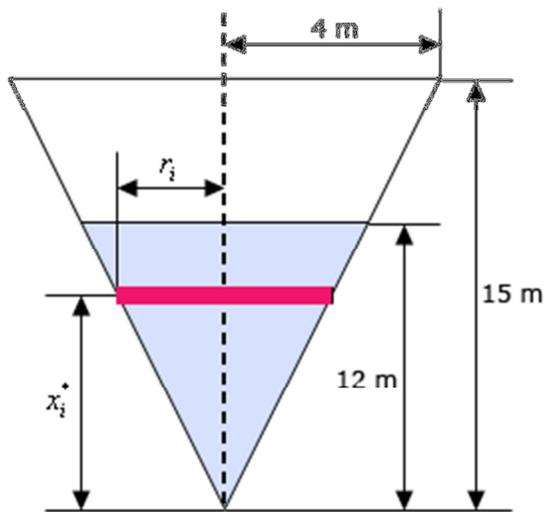
The red strip in the sketch represents the “cylinder” of water in the  $i^{\text{th}}$  subinterval. A quick application of similar triangles will allow us to relate  $r_i$  to  $x_i$  (which we’ll need in a bit) as follows
